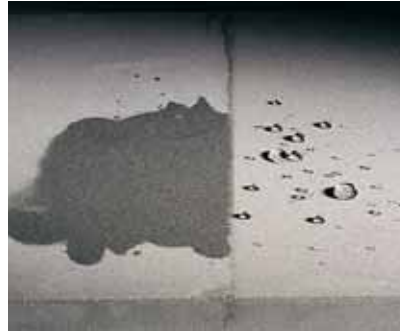
Half of this porous stone has been treated with Fila products while the other half has not. On the treated side (right), the drip-effect of water is visible. On the untreated side the water has penetrated the floor.
